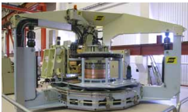
Figure A15: The Canister Laboratory's equipment for development of friction stir welding.
