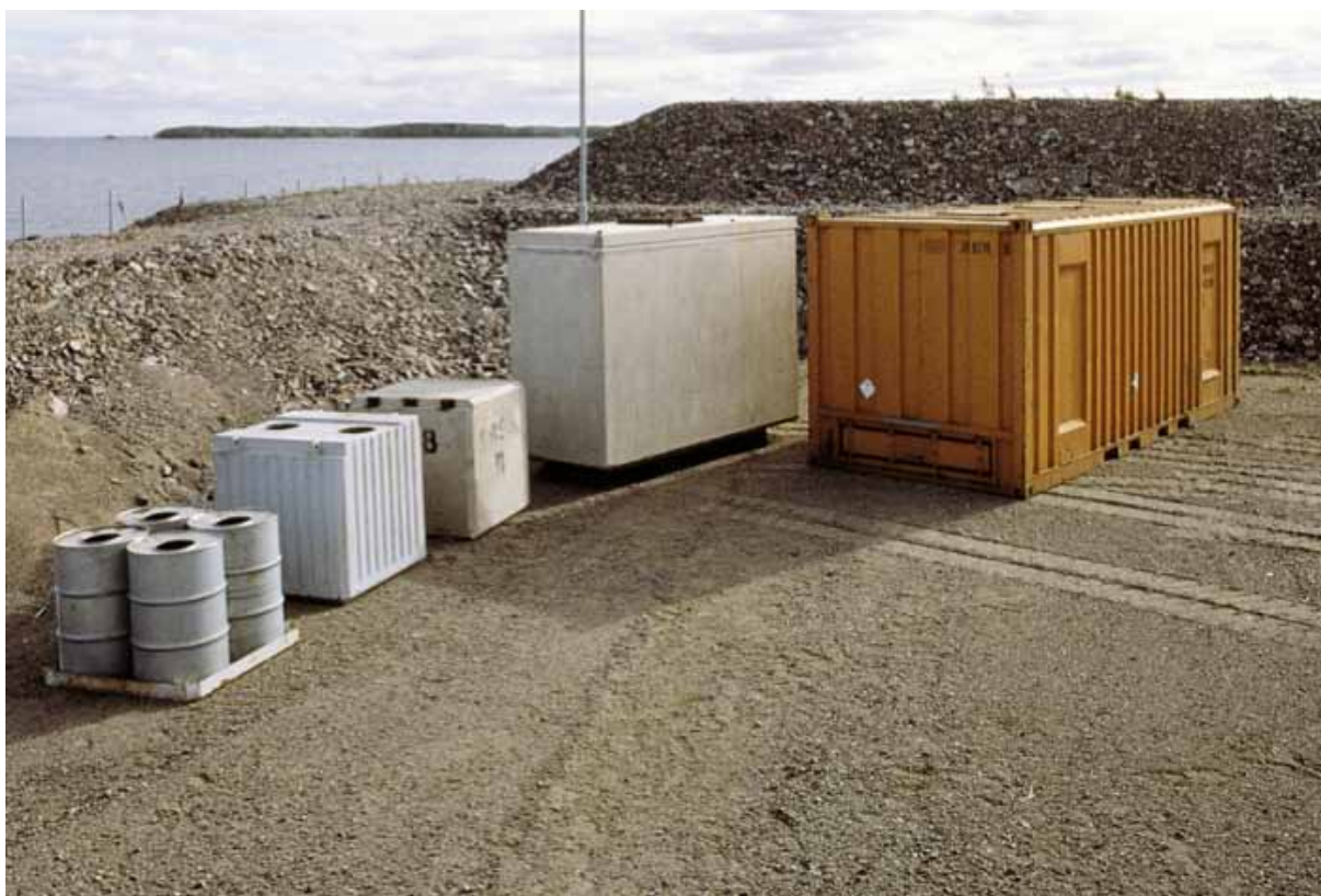
Figure D1: Standard packages for short-lived LILW used in Sweden.
