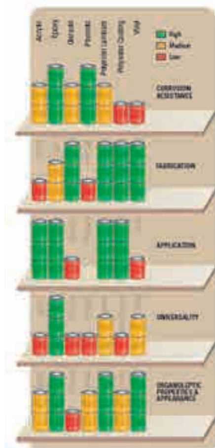
Diagram 6.1 Qualitative rankings of major resin types in terms of technologic feasibility and consumer acceptance
