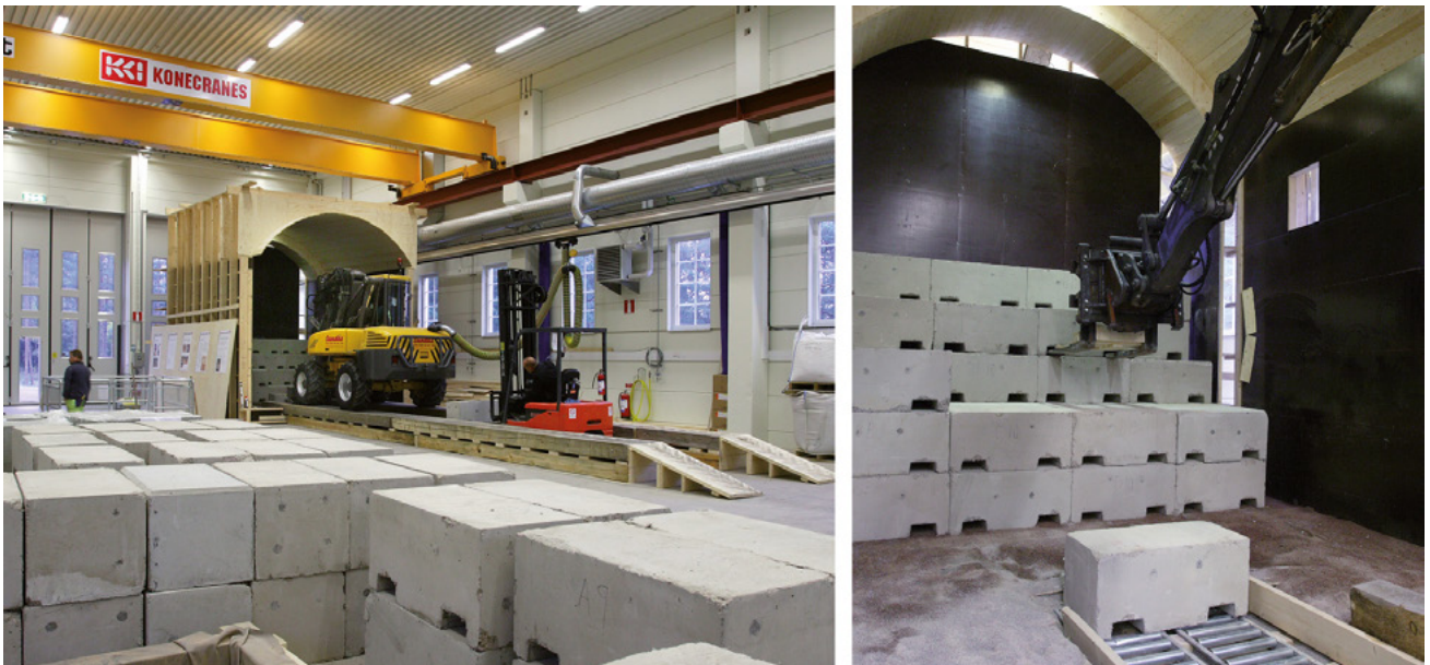
Figure A15 The Multi-purpose Test Facilities at Äspö. The photo shows the testing of a self-positioning robot for backfilling a deposition tunnel with bentonite blocks.
