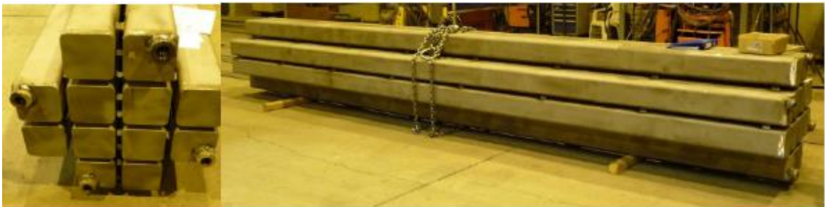
Figure 4 The steel cassette construction for BWR insert.[11]
