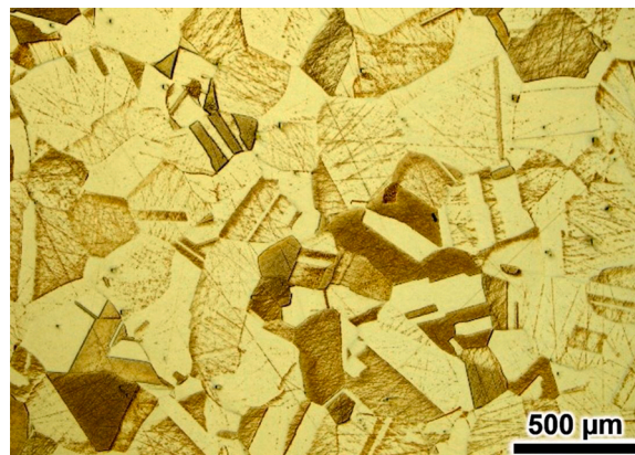
Fig. 1. Optical micrograph of an etched copper sample showing typical microstructure (large grains and annealing twins) of canister material.
