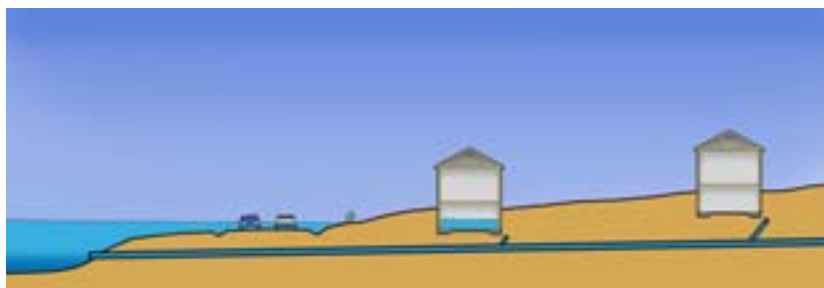
Figure 4.35 Very high water levels with backed up service pipes and flooded basements
