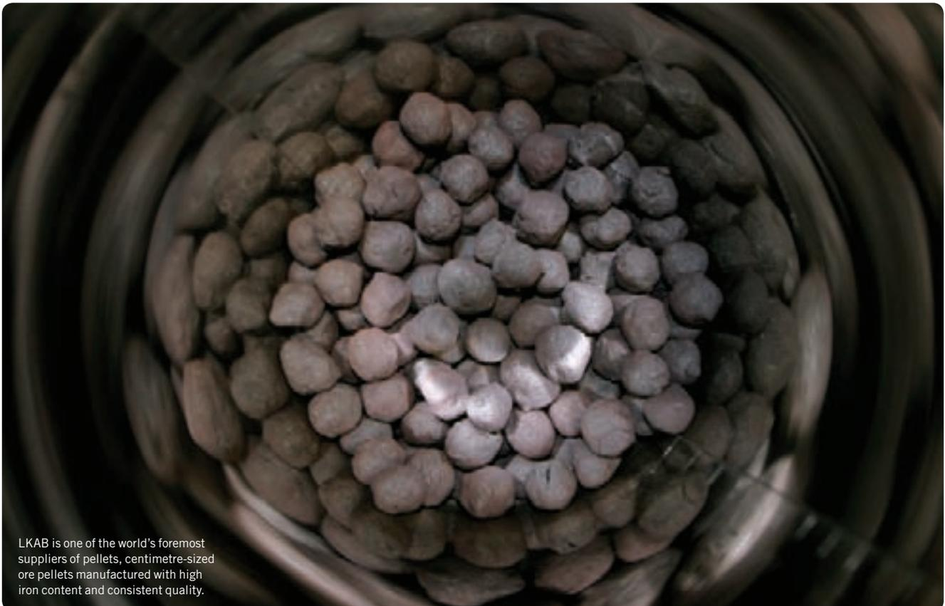
LKAB is one of the world's foremost suppliers of pellets, centimetre-sized ore pellets manufactured with high iron content and consistent quality.
